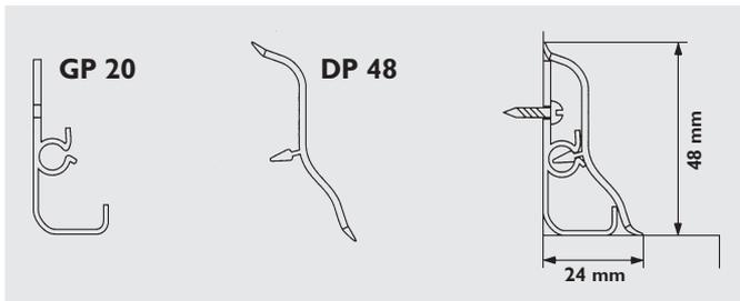
The SL 48 skirting consists of a base profile (GP 20) and a decorative profile (DP 48), as well as the relevant corner pieces, end caps and connectors.
